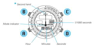
Second hand indicates the elapsed seconds for the first 60 seconds and stays at the "0" position thereafter. (Hour and Minute hands indicate the current time)
